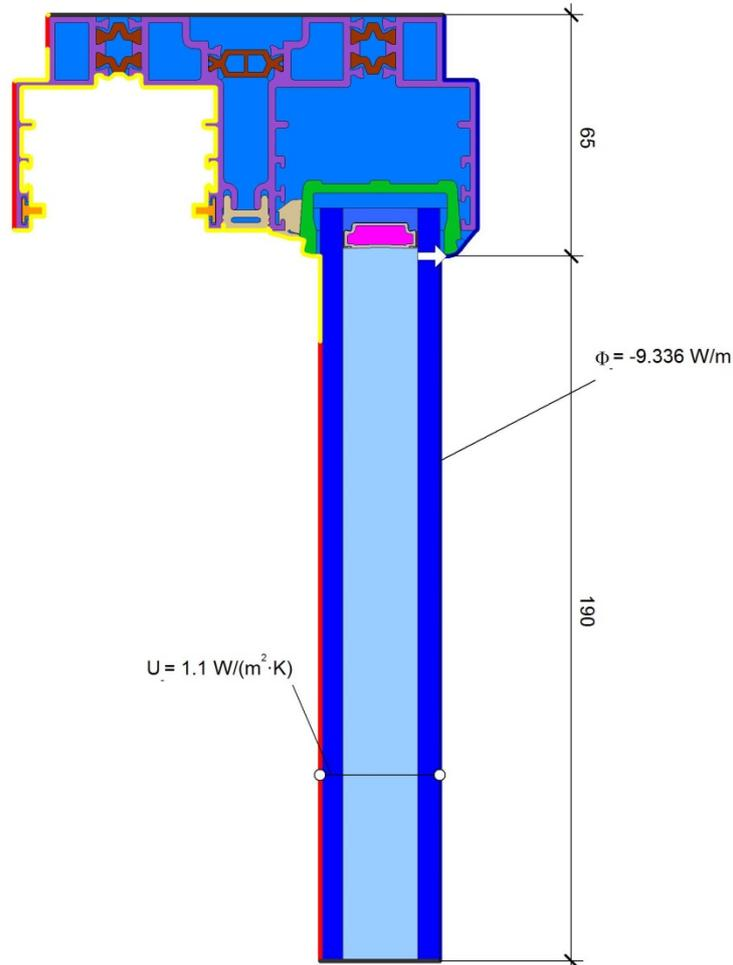
$$\psi = \frac{\Phi}{\Delta T} - U_g \cdot b_g - U_f \cdot b_f = \frac{9.336}{20.000} - 1.100 \cdot 0.190 - 3.277 \cdot 0.065 = 0.045 \text{ W/(m}\cdot\text{K)}$$
