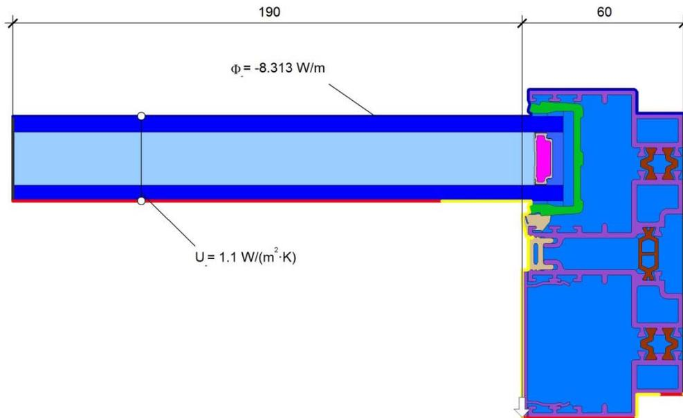
$$\psi = \frac{\Phi}{\Delta T} - U_g \cdot b_g - U_f \cdot b_f = \frac{8.313}{20.000} - 1.100 \cdot 0.190 - 2.673 \cdot 0.060 = 0.045 \text{ W/(m} \cdot \text{K)}$$
