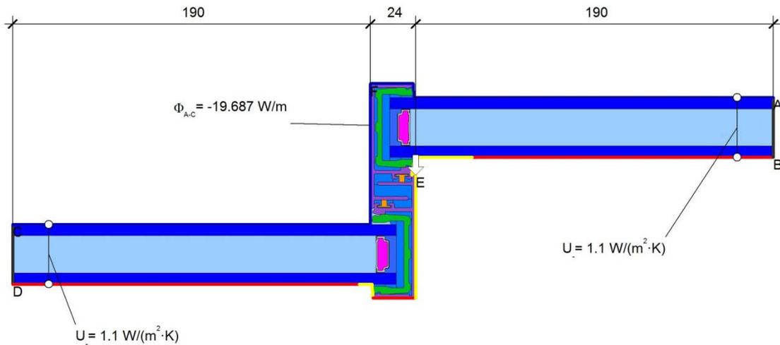
$$\psi_{A-E-C} = \frac{\Phi}{\Delta T} - U_1 \cdot b_1 - U_2 \cdot b_2 - U_3 \cdot b_3 = \frac{19.687}{20.000} - 1.100 \cdot 0.190 - 19.555 \cdot 0.024 - 1.100 \cdot 0.190 = 0.097 \text{ W/(m}\cdot\text{K)}$$
