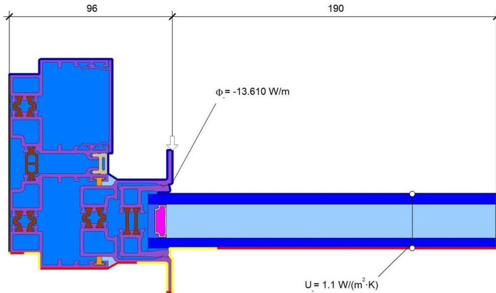
$$\psi = \frac{\Phi}{\Delta T} - U_g \cdot b_g - U_r \cdot b_r = \frac{13.610}{20.000} - 1.100 \cdot 0.190 - 4.439 \cdot 0.096 = 0.047 \text{ W}/(\text{m} \cdot \text{K})$$
