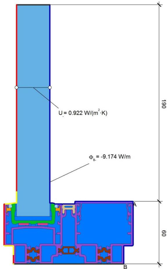
$$U_{fA,B} = \frac{\frac{\Phi}{\Delta T} - U_p \cdot b_p}{b_f} = \frac{\frac{9.174}{20.000} - 0.922 \cdot 0.190}{0.060} = 4.691 \text{ W}/(\text{m}^2 \cdot \text{K})$$
