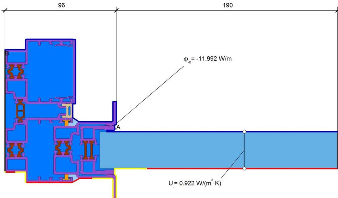
$$U_{f,A,B} = \frac{\frac{\Phi}{\Delta T} - U_p \cdot b_p}{b_f} = \frac{\frac{11.992}{20.000} - 0.922 \cdot 0.190}{0.096} = 4.439 \text{ W/(m}^2 \cdot \text{K)}$$
