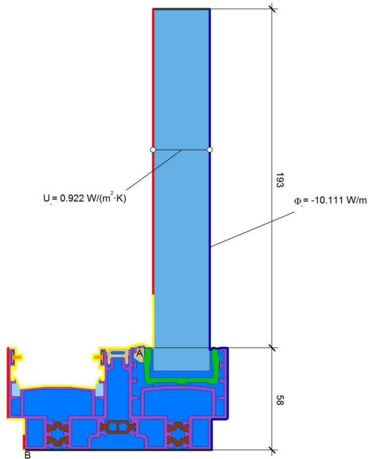
$$U_{fA,B} = \frac{\frac{\Phi}{\Delta T} - U_p \cdot b_p}{b_f} = \frac{\frac{10.111}{20.000} - 0.922 \cdot 0.193}{0.058} = 5.655 \text{ W/(m}^2 \cdot \text{K)}$$
