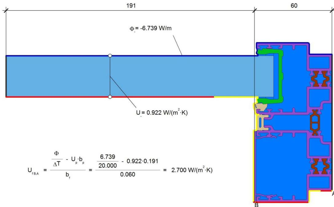
$$U_{f,BA} = \frac{\frac{\Phi}{\Delta T} - U_p \cdot b_p}{b_f} = \frac{\frac{6.739}{20.000} - 0.922 \cdot 0.191}{0.060} = 2.700 \text{ W/(m}^2\cdot\text{K)}$$
