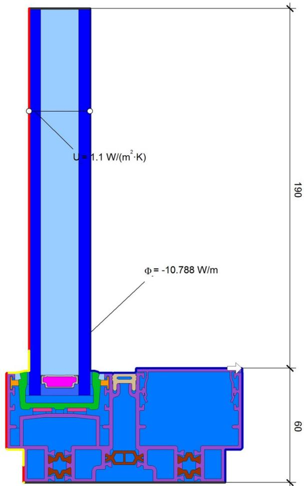
$$\psi = \frac{\Phi}{\Delta T} - U_g \cdot b_g - U_f \cdot b_f = \frac{10.788}{20.000} - 1.100 \cdot 0.190 - 4.667 \cdot 0.060 = 0.048 \text{ W/(m}\cdot\text{K)}$$
