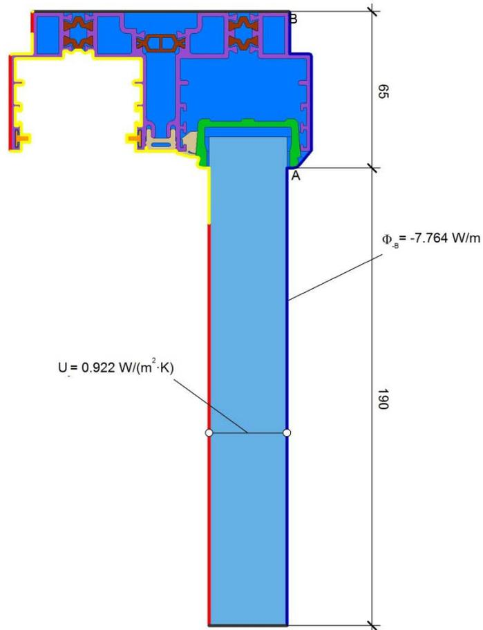
$$U_{fA,B} = \frac{\frac{\Phi}{\Delta T} - U_p \cdot b_p}{b_f} = \frac{\frac{7.764}{20.000} - 0.922 \cdot 0.190}{0.065} = 3.277 \text{ W/(m}^2 \cdot \text{K)}$$
