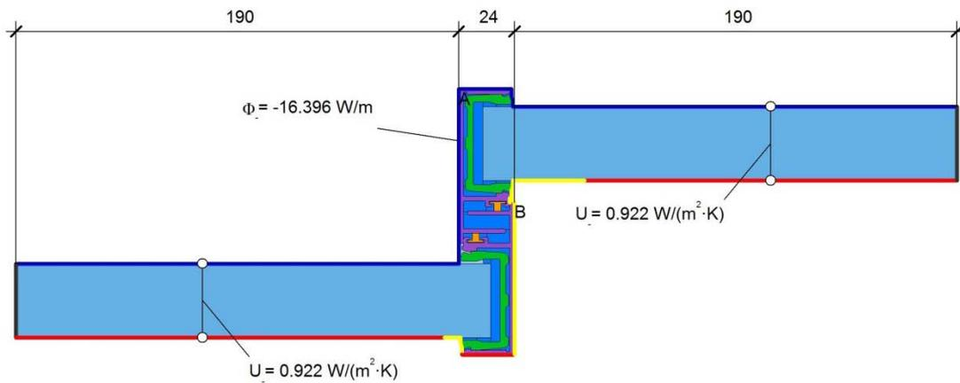
$$U_f = \frac{\frac{\Phi}{\Delta T} - U_{p1} \cdot b_{p1} - U_{p2} \cdot b_{p2}}{b_f} = \frac{\frac{16.396}{20.000} - 0.922 \cdot 0.190 - 0.922 \cdot 0.190}{0.024} = 19.555 \text{ W/(m}^2 \cdot \text{K)}$$
